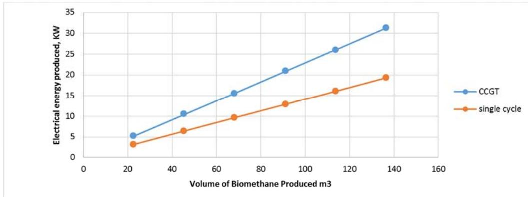
Figure 5. Electrical energy Vs volume of biomethane yield for human waste decomposition per day.
