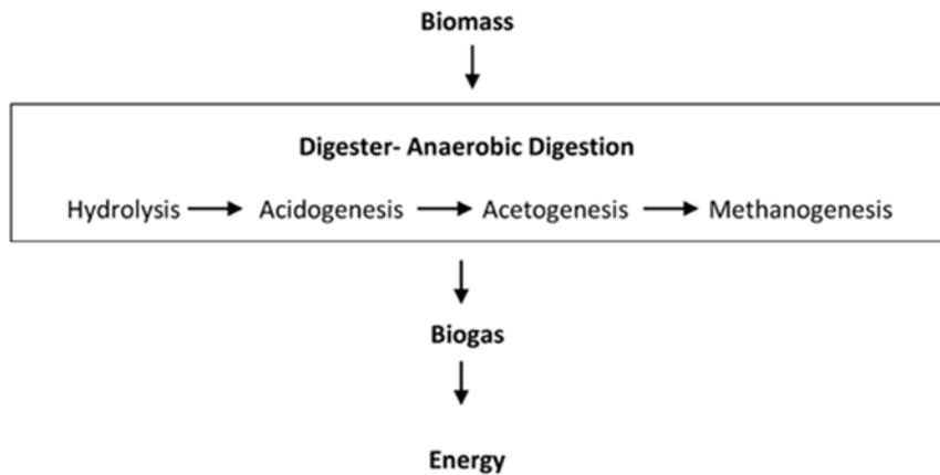
Figure 1. Processes in anaerobic digestion of biomass.
